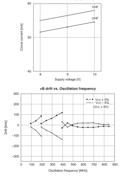
Circuit current vs. Supply voltage
